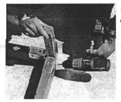
Check that the base is square by measuring from corner to corner in both diagonal directions. If the measurements are not equal, push on the longer dimension until they are equal.
