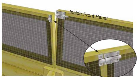
**12.** Attach Barrel Bolt to Inside of Front Panel framing. Pre-drill shallow 1/8" holes to prevent wood from splitting. Do a dry run first to confirm screw alignment before completely securing.
