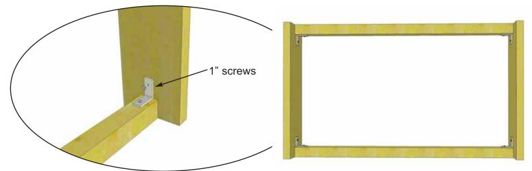
**10.** Locate Brackets (4). Position Brackets in each corner and secure with 2 - 1" screw per Bracket.
