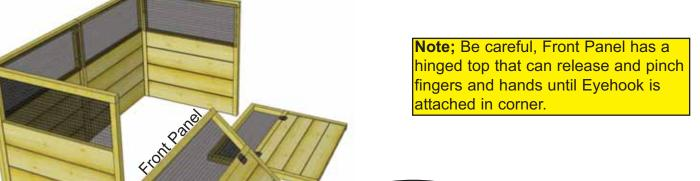
**6.** Align and attach Front Panel - **Part B** to Side Panel with 3 - 2 1/2". Align panel framing together as **Step 2**. Screw only into Front Panel framing below the screen hinged top.
