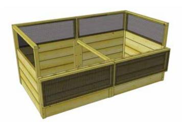
**13.** To access your Raised Garden Bed, open the Barrel Bolt and Eyehook in corner(s) to release the screened hinged panel. Be sure to close when your finished to keep dogs and pesky critters out!
