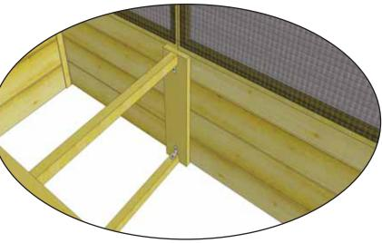
**11.** Lift and position completed Bed Rib between Front and Rear Panels at the mid point. Align with bottom of panels and centered on framing. Secure with 6 - 2" screws per plate. **Important-** be sure to screw into panel framing.
