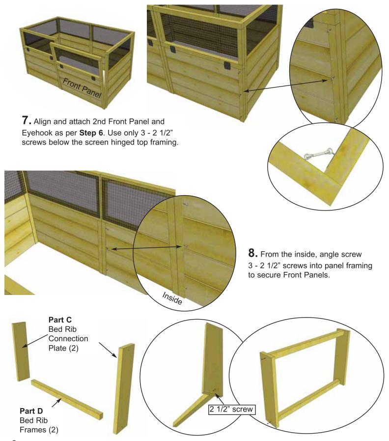
**9.** Locate Bed Rib Connection Plates (2) - **Part C** and both Bed Rib Frames (2) - **Part D**. On a level flat surface, screw Connection Plate and Frame together with 1 - 2 1/2" screw. Align so Plate and frame are flush at bottom. Complete both sides. Attach 2 Bed Rib Frames as illustrated above.
