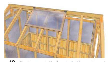
**49.** Standing on a ladder from the inside, position and attach **Part Z - Vent Hinged Window** to Ridge Board. Prior to attaching, confirm Window can move up and down freely. Attach with 3/4" Black screws.
