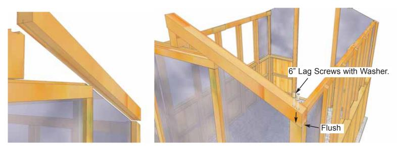
**33.** Position Rafter so end is flush with Corner Post and Outside Polygal Angle Cut Window slides into dado cut of Rafter. When orientated correctly, start 2 - 6" Lag Screws with 3/8" Washer with a hammer and tighten with 9/16" socket.
