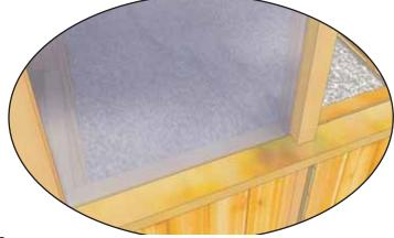
**25.** Slide **Window** down into the dado cut of the Top Cap.
