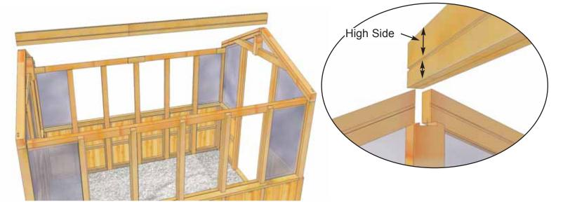
**41.** Before installing completed Ridge Board, note that dado cut is off center. Orientate Ridge Board with high side to top before lifting. See illustration above.
