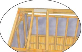
**46.** Install second **Part U - Roof Rafter using Rafter Template Spacer.** Align Spacer tight against Rafter's 2x3 edge. Position Rafter so dado cut of Ridge Board is aligned with gap in Rafter and tight against 2x3 edge of new Rafter. Attach as per **Step 45**.
