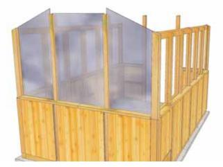
**27.** Locate a second **Part K - Outside Angle Cut Polygal Window - 26 1/2" wide.** Position as per **Step 24-25**.
