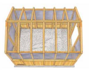
**48.** Install Center Rafters to complete Rafter section as illustrated above and to the right as per **Steps 45 & 46.** Confirm Center Rafter location using **Part Z** or **V**. Adjust if necessary.
