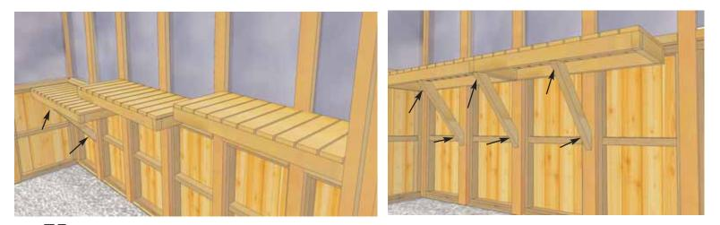
**75.** Position Potting Shelf Support against Post and under Shelf framing. Level Shelf and attach Support with 2 - 3" screws. Complete Shelving and Supports for side.
