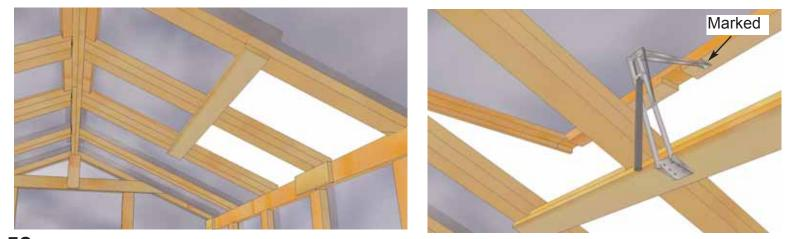
**58.** Complete both Supports. Locate both **Heat Activated Hinges.** Hinged Window will be marked for correct location for Hinge. Heat Activated Hinge will require a basic assembly. Follow Manufacturer's directions. Attach with Manufacturer's Hardware supplied. **Phillips Head Driver will be required.**
