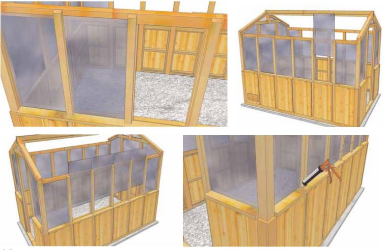
**44.** Once all Side Windows are installed. Caulk Window / Wall Top Cap seam. Work around the entire Greenhouse. Gaps in Wall Top Caps can also be caulked at this time. No need to caulk sides or top at this time.
