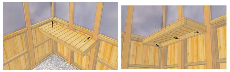
**74.** Locate Parts MM and NN - Potting Shelves - 16" x 45 3/8" and Potting Shelf Supports - 1 1/2" x 2 1/2" x 20 1/2". With helper holding Shelf just under the Top Wall Cap, screw to wall from underneath with 3 - 3" screws as shown above.
