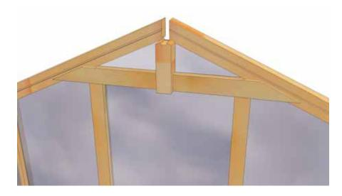
Rear Wall shown with Rafters, King Stud and Gable Support Frame configured correctly.
