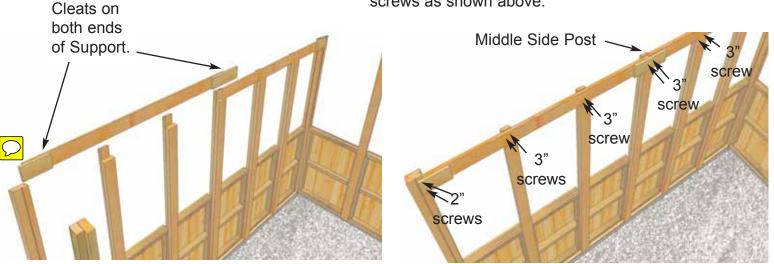
**17.** Position and attach Side Top Support with Cleats on both ends as per **Step 16**. Attach Corner Post(s) End first with 2 - 2<sup>°</sup>. Align Supports equally on middle Side Post and attach with 2 - 3<sup>°</sup> screws. Attach remaining interior Posts with 2 - 3<sup>°</sup> screw as shown above.
