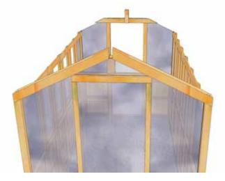
**37.** When Rafter is orientated correctly, start 2 - 6" Lag Screws with Washers with a hammer and tighten with 9/16" socket. From the inside, attach Gable Support Frame to Rafters with 4 - 1 1/4" screws. See illustration below.
