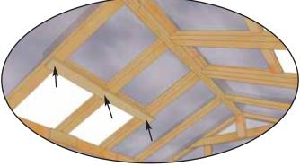
**57.** Locate and attach **Part V - Inside Vent Framing Supports - 3/4" x 2 1/2" x 49"** with 6 - 2" screws. Position parallel with Hinged Window.
