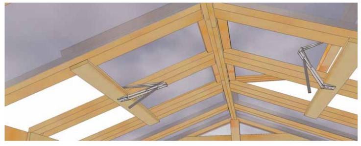
**Important-** Heat Activated Hinges will open only after the Greenhouse reached an inside temperature of approximately 75 degrees Fahrenheit. Make sure Hinged Windows open easily and do not stick. We recommend purchasing a thermometer once the Greenhouse is complete. Please monitor Heat Activated Hinges to confirm they open and are functioning correctly.
