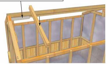
Spacer tight against Outside Rafter Spacer tight against 2x3. Align dado cuts with gap in Rafter. and Align dado cuts with gap in Rafter. Flush
