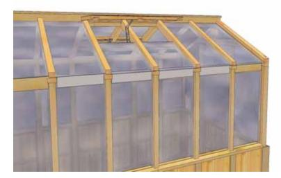
**72.** Position 19 1/8" Soffits underneath remaining Roof Window and attach as per **Step 71.**
