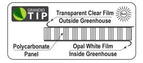
Make sure the UV coated side of the panel faces outward as indicated on the panels. Avoid placing the polycarbonate panels in the sun or near plants until fully assembled.
