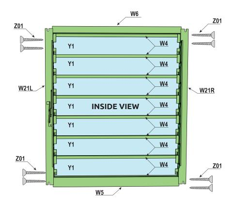
**NOTE:** Louver may be installed during construction or on a fully assembled Grandio Greenhouse. If installing during construction, it is recommended to place the louver while installing the panels in your desired location. If installing after construction, you will need to cut the panel of choice out of the greenhouse. A utility blade or jigsaw is recommended.
