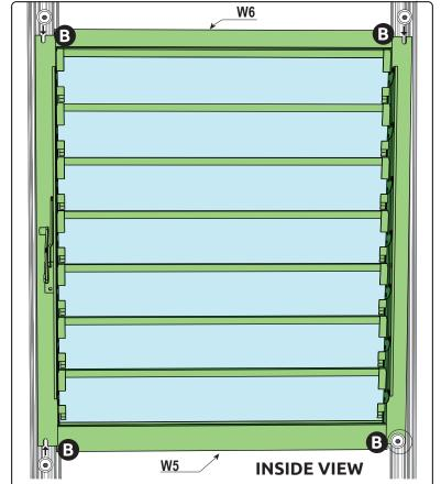
**Note:** Polycarbonate panel will sit inside the **W5** or **W6** extrusion one end may fit snug to the greenhouse extrusion, or both top and bottom may have panels. It will depend on placement how you will cut your panels.
