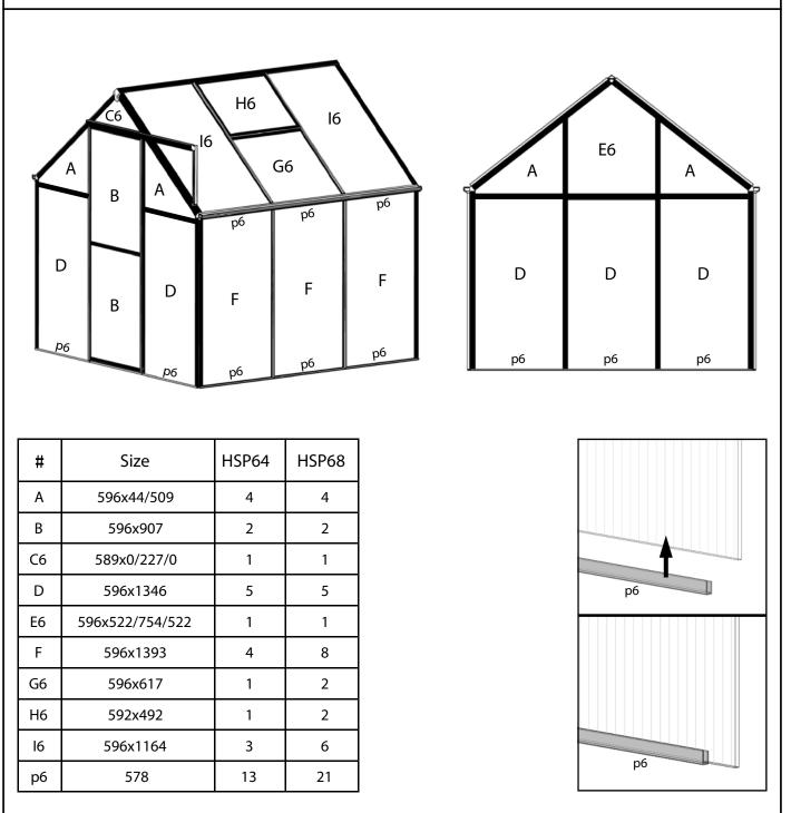
This page shows the positioning of the polycarbonate panels for the front and rear gable as well as the roof and the sides. It also indicates where the parts #p6 is used. When fitting parts #p6 on the ends of the panels, try using a narrow piece of bar soap through the part first. It will allow it to slide on much easier. #p6 must be fitted on both ends of polycarbonate in advance before polycarbonate be inserted into aluminum frame.
